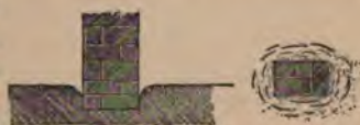
FIG. 52. — Heavy post sunk deeper into the ground during the Charleston earthquake of August 31, 1886 (after Dutton).
